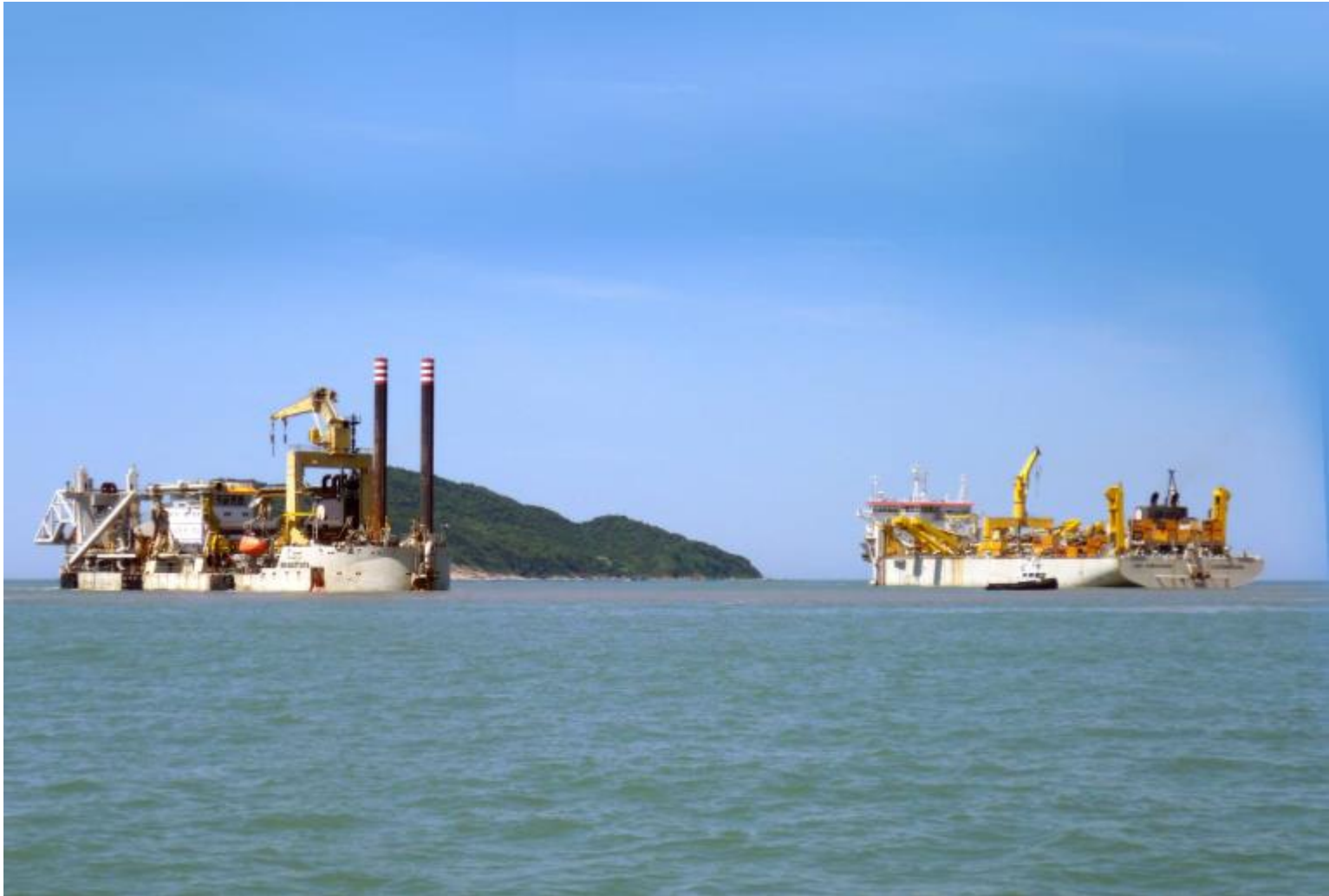
Vietnam - Trailing Suction Hopper Dredger Leiv Eiriksson and Cutter Suction Dredger Ibn Batutta dredging and reclaiming for the Ha Tinh Steel Mill Complex-2000ha reclamation
